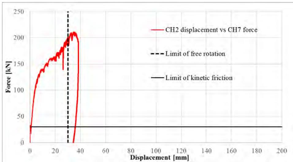
Figure 10. CH2 measurement
