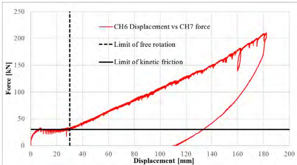
Figure 7. CH6 measurement
