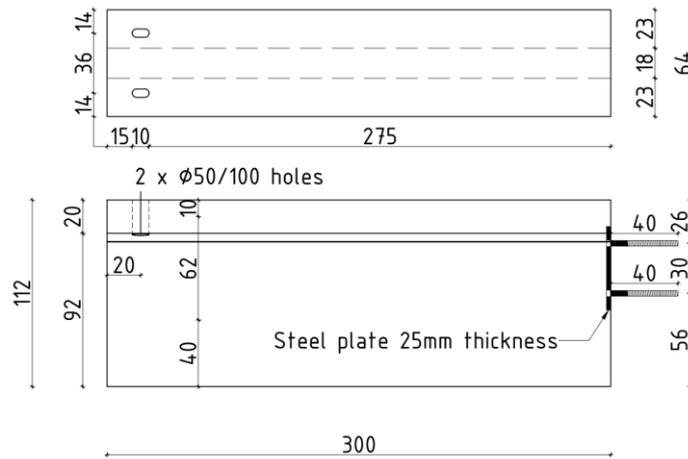
Figure 4. Beam dimensions
